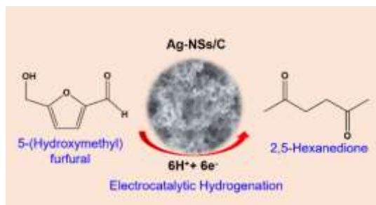
Figure1: Schematic representation of the electrocatalytic hydrogenation of HMF to HD
